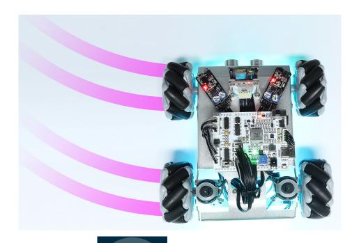
• Similarly, if you slide the Q widget clockwise, the Zeus Car will drift to the left and stop in the current position.
