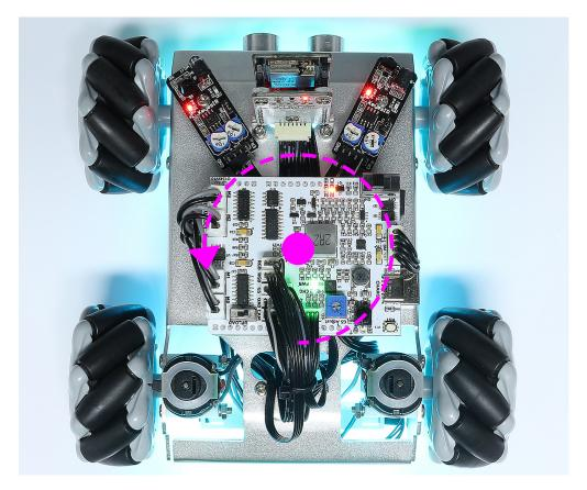
• turn right: This command will make the car turn  $45^{\circ}$  to the right with the body as the center, and again will move forward or stop depending on the previous state.
