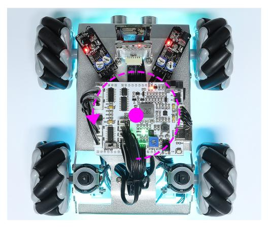
• turn right: This command will make the car turn  $45^{\circ}$  to the right with the body as the center, and again will move forward or stop depending on the previous state.
