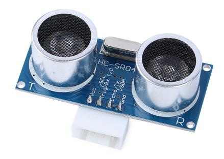
TRIG: Trigger Pulse InputECHO: Echo Pulse Output
