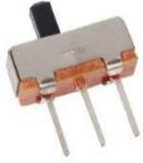
A slide switch, just as its name implies, is to slide the switch bar to connect or break the circuit, and further switch circuits. The common-used types are SPDT, SPTT, DPDT, DPTT etc. The slide switch is commonly used in low-voltage circuit. It has the features of flexibility and stability, and applies in electric instruments and electric toys widely.
