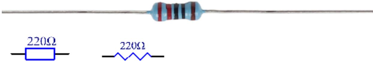
When using a resistor, we need to know its resistance first. Here are two methods: you can observe the bands on the resistor, or use a multimeter to measure the resistance. You are recommended to use the first method as it is more convenient and faster. To measure the value, use multimeter.
