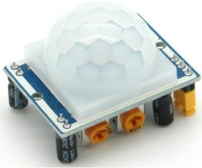
After the sensing module is wired, there is a one-minute initialization. During the initialization, module will output for 0~3 times at intervals. Then the module will be in the standby mode. Please keep the interference of light source and other sources away from the surface of the module so as to avoid the misoperation caused by the interfering signal. Even you'd better use the module without too much wind, because the wind can also interfere with the sensor.
