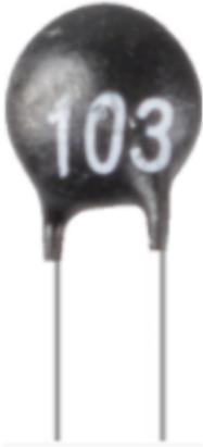
The principle is that the resistance of the NTC thermistor changes with the temperature of the outer environment. It detects the real-time temperature of the environment. When the temperature gets higher, the resistance of the thermistor decreases. Then the voltage data is converted to digital quantities by the A/D adapter. The temperature in Celsius or Fahrenheit is output via programming.
