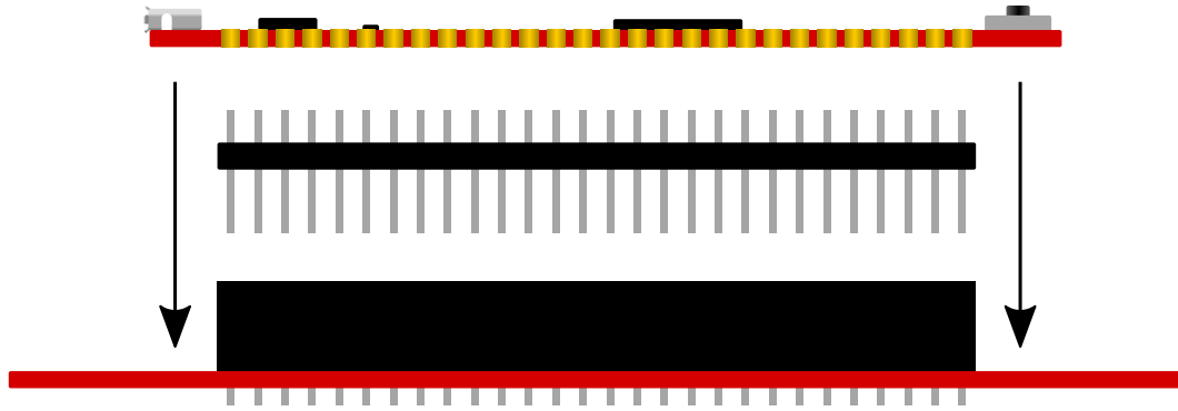
Figure 5-1. Connecting Curiosity Nano Board to Base Board Using Pin Headers
